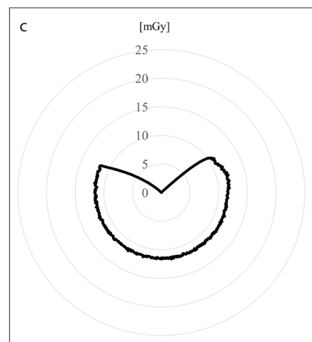
Figure 5. a–c. Output-dose profile of the three scanning methods. The figure shows the output-dose profile obtained with each scanning method. The plots show the superposition of each of the five measurements. Panels (a), (b), and (c) correspond to the output-dose profiles of OS, OS_{Bismuth} , and PEM, respectively. In panels (a) and (b), dose increased when exposure overlap associated with the fan beam angle occurred. Additionally, the dose increases were observed at an arbitrary position because the start position of the tube rotation was not fixed. The output-dose profile of the PEM, shown in panel (c), demonstrates a decrease in the dose above the gantry.
